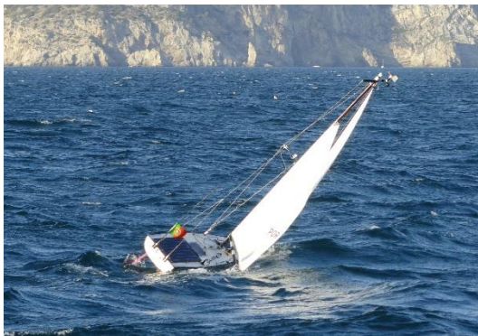
FASt Autonomous Sailboat, Length 2.5m, University of Porto / INESC TEC
